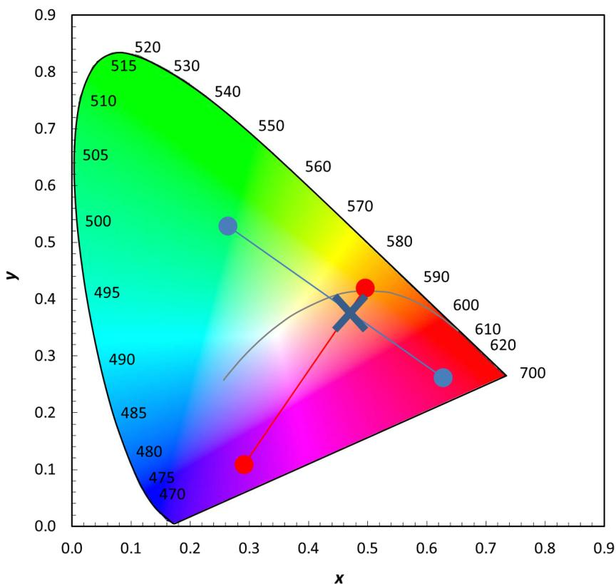
Figure 2. Chromaticity diagrams, such as the CIE 1931 ( $x, y$ ) chromaticity diagram shown here, are used to provide a numerical specification for the color of light. The colored background is for visual reference only, as chromaticity diagrams do not account for lightness. The numbers around the outside indicate the wavelength of monochromatic light at the coordinate, in nanometers. Colors outside the shaded area are not visible to humans.
